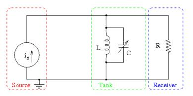
(a) (5 pts) Show that when  $\omega \approx 1/\sqrt{LC}$  the impedance of the parallel *LC* combination is very large, such that the signal is passed to the receiver (resistor *R*). On the hand, show that when  $\omega$  is far from  $1/\sqrt{LC}$ , the impedance of the tank circuit is very low such that the signal is not passed to the receiver.
